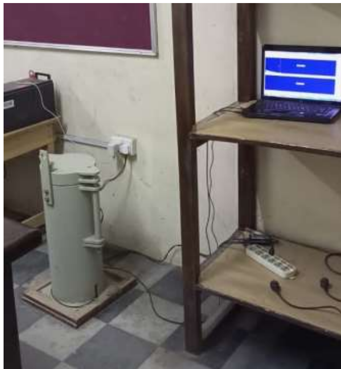
Plate 2: The gamma-ray spectrometer setup showing (a) open lead shield revealing top of the Bicron NaI(Tl) detector (b) and closed lead shield enclosing the Bicron 2"x2" NaI(Tl)
